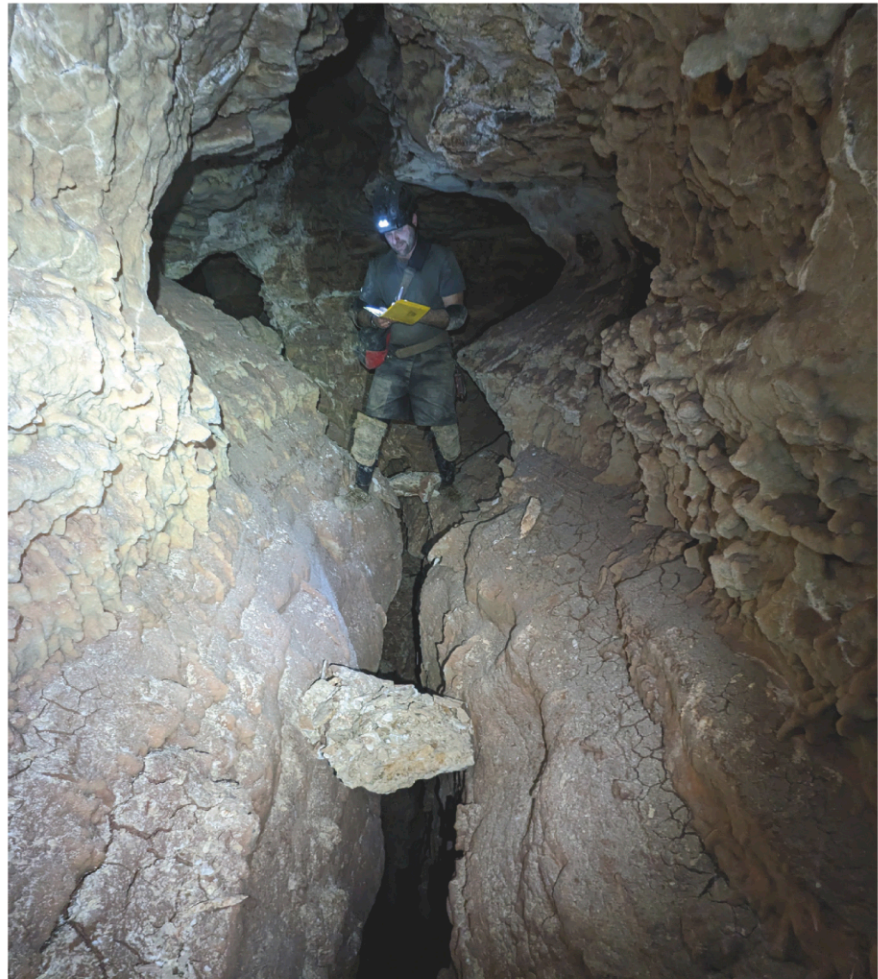
Volunteer cave explorer Dan Austin sketching a passage of Jewel Cave. Using coordinates to draw a survey line in the book, Austin draws the cave walls around the line to represent the cave walls around him, adding additional notes as needed. Image credit: NPS
